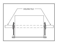
c. Compress the spring clips on the back box and push it through the hole, until the clips spring back. Tighten the screws until you hear a clicking noise.
